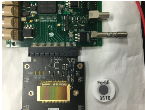
Figure 37: Source (Fe55) used in the experiment.
