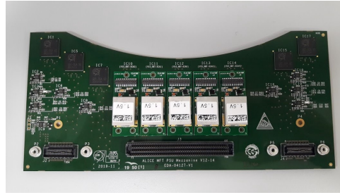
FIGURE 2.10: PSU mezzanin board
