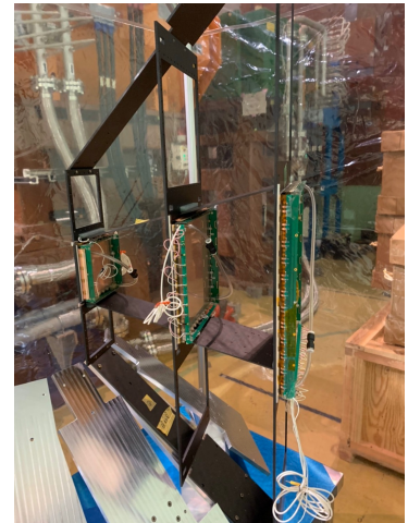
Figure 3.13: Conceptual diagram of GTR (left) and the CFRP frame and the provisionally mounted GTR are shown (right). The black frame is the CFRP frame, and from left to right on the middle tier are the GTR100, GTR200, and GTR300 [36].
