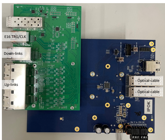
Figure 4.8: GBTxEMU and FMC board.
